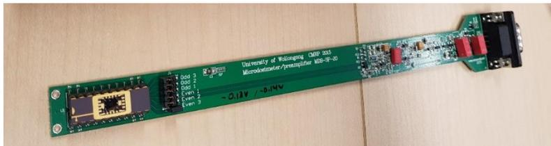
Diamond sensors are compatible with microPlus probe developed @ UoW for Si microdosimeters
