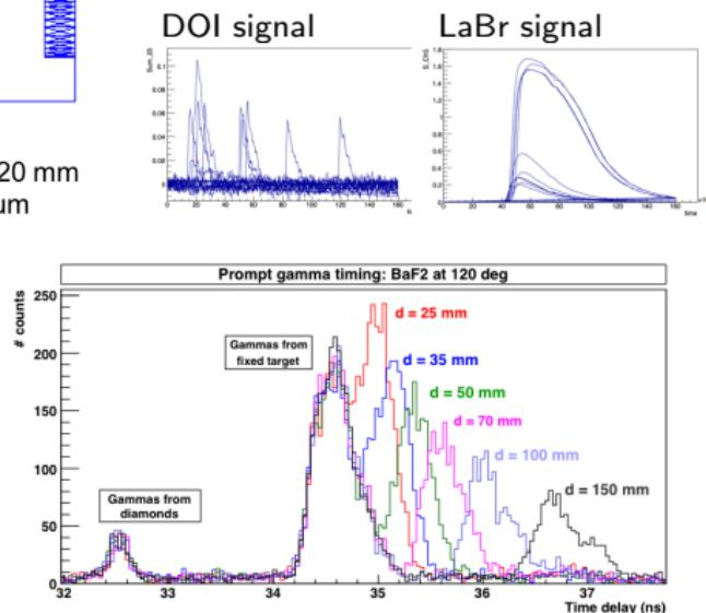
**Aim:** exploit the-ultra fast coincidence time to detect range variations due to target heterogeneities
