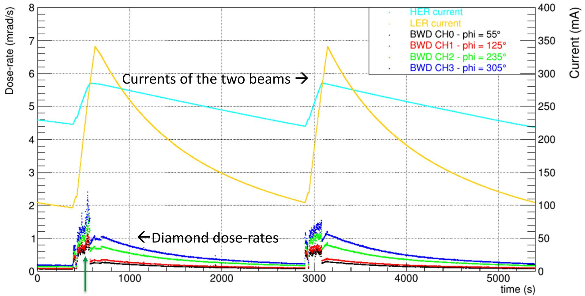
The spikes from diamonds are due to transient increases of radiation during injections
