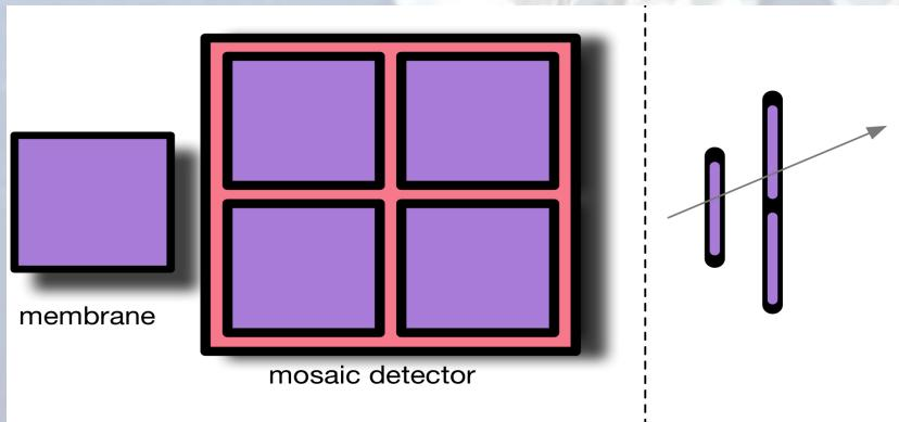
membrane is the thin detector of few um thickness
