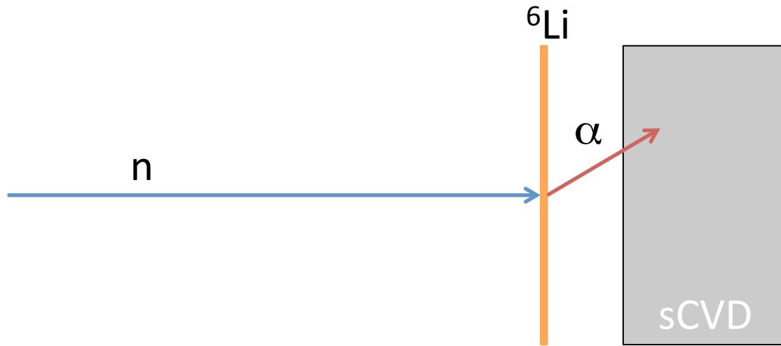
External converter needed:  ${}^6\text{Li}$ ,  ${}^{10}\text{B}$ ,  ${}^{235}\text{U}$ , ...
