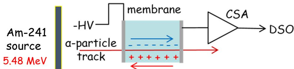
no multiplication up to  $150 \text{ V}/\mu\text{m}$  ( $\sim 500\text{V}, 1.5 \text{ MV/cm}$ ) for 5.5 MeV  $\alpha$ -particles
