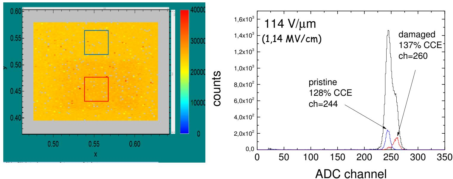
Complete recovery of CCE possible! (avalanching higher in damaged area)
