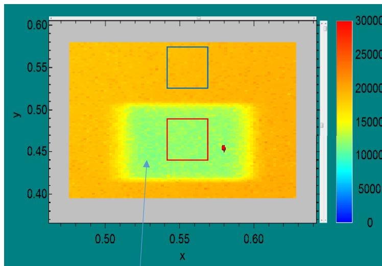
Region damaged with  $1 \times 10^{11}$  O (18 MeV) ions/cm<sup>2</sup>
