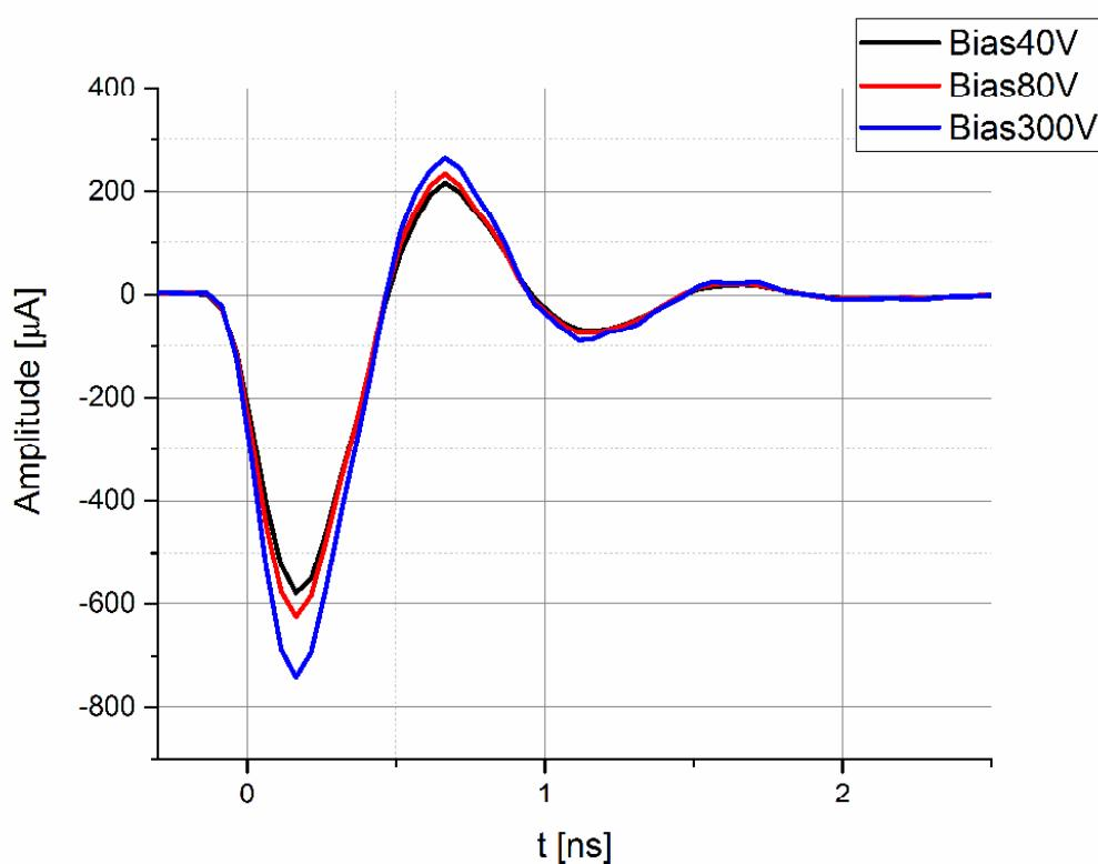
Transient in  $3.5 \mu\text{m}$  at  $> 30 \text{ V}/\mu\text{m}$
