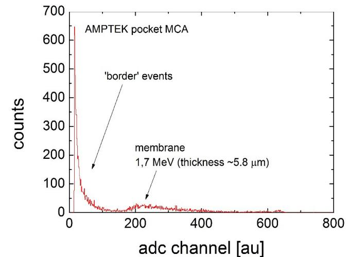
About 100 MeV deposited in the membrane
