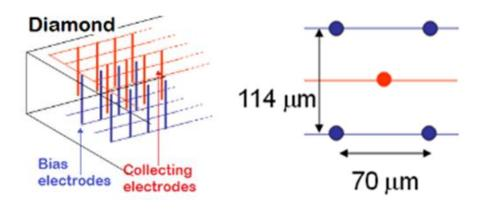
The resulting structure has arrays of graphitic columns of about 10  $\mu$ m in diameter forming cells of 114 x 70  $\mu$ m with a thickness of 0.5 mm for a total of 275 cells with a single cell sensitive volume of 0.004 mm<sup>3</sup> and a total diamond sensitive volume of about 1.1 mm<sup>3</sup>.
