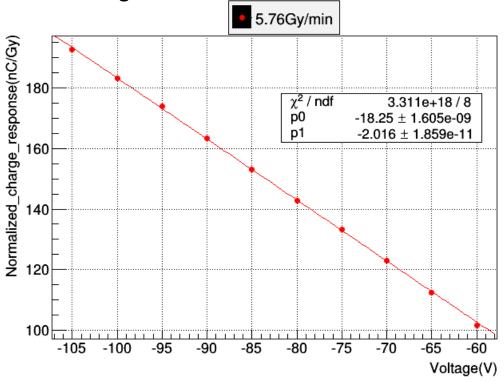
There are 275 3D single cells, each one with a 0.004 mm<sup>3</sup> sensitive volume and a spatial resolution of 0.008 mm<sup>2</sup>. At -80V the sensitivity
