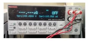
The detector was biased with a Keithley source meter 2410 and the output current is obtained by reading in parallel all the collecting graphitic columns.
