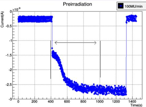
The dose necessary for pumping the diamond was about 820 MU.
