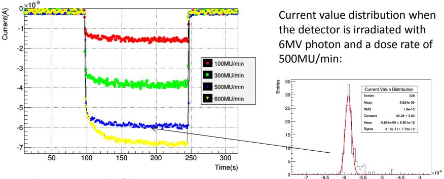
The output signal of the detector is an electric current so in principle it measures dose rates.
