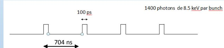
A 8.5 keV photon focused micro-beam with a well-defined time structure was used at the ESRF.
