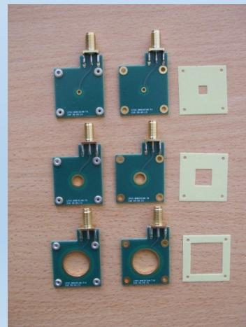
Diamond  $0.45 \times 0.45 \text{ cm}^2 \times 500 \mu\text{m}$  sc-CVD E6
