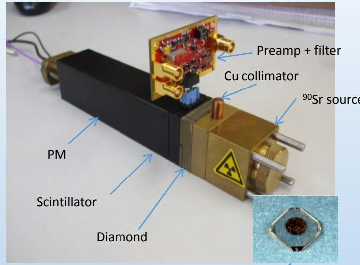
Triggering on high energy electrons (scintillator behind diamond)
