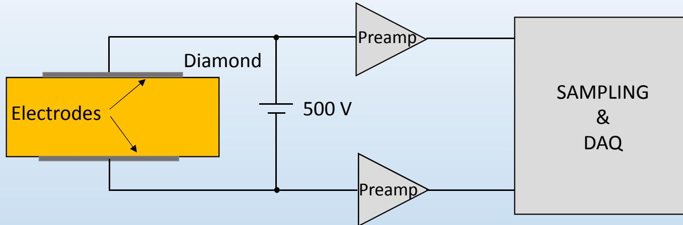
Diamond  $0.45 \times 0.45 \text{ cm}^2 \times 500 \mu\text{m}$  sc-CVD E6
