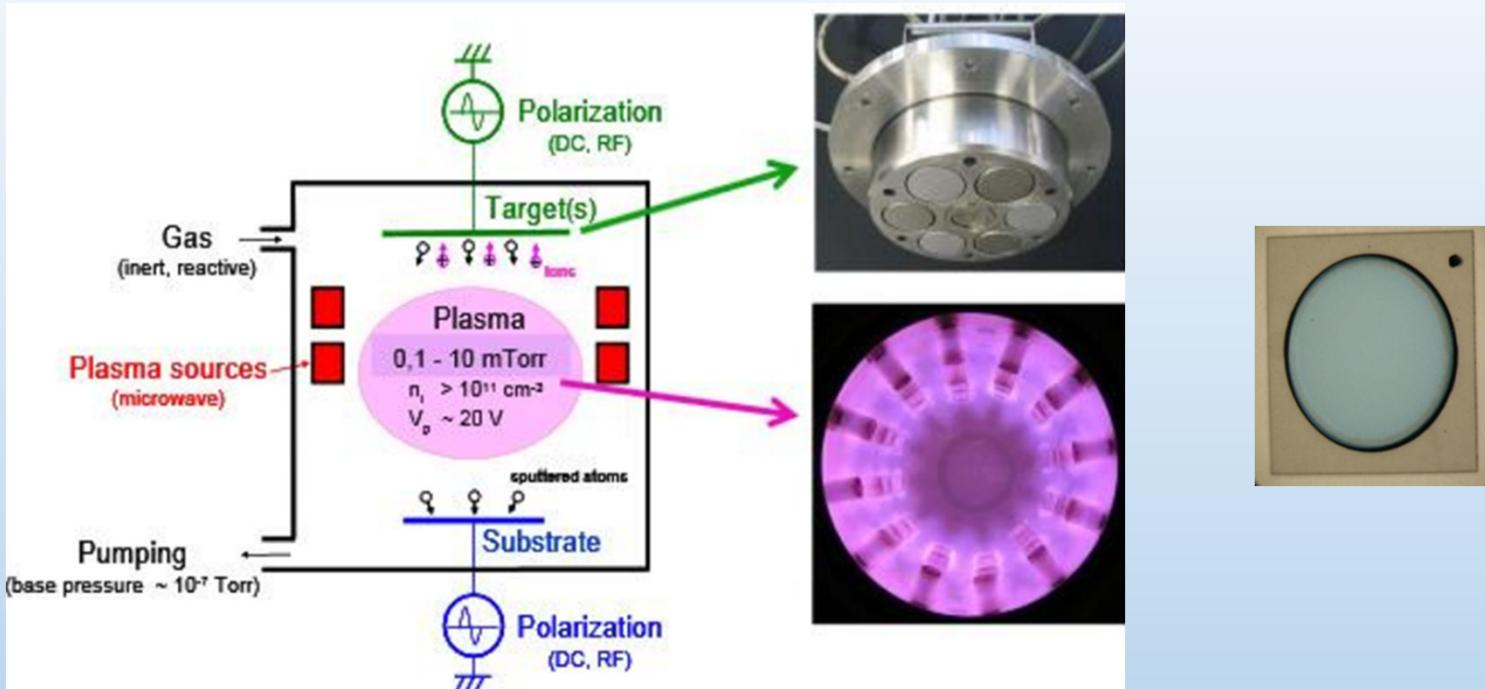
The crystal surface preparation and metal deposition is performed by a sequential plasma process consisting in two steps of reactive plasma processing followed by plasma-assisted sputtering
