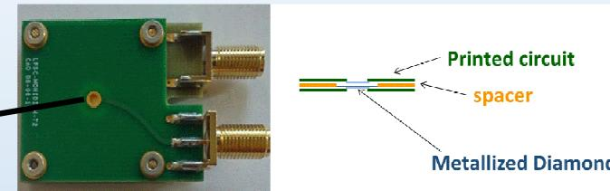
➤ Final detector : 15 x 15 cm<sup>2</sup> mosaic arrangement of stripped sensors => channels >10<sup>3</sup>
