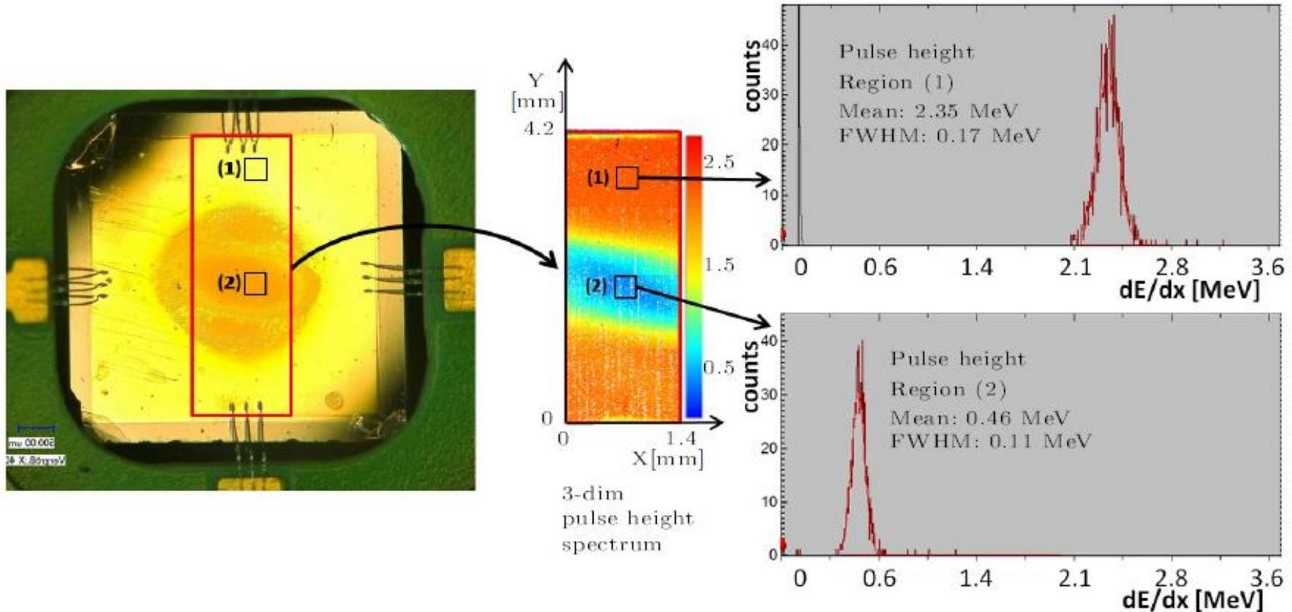
→ pulse height spectrum reduced by a factor of 5.1 at absorbed dose of about 87 MGy
