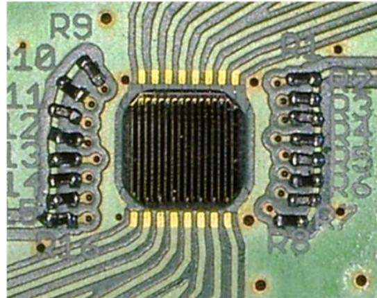
ADC scan → radiation damage pattern
