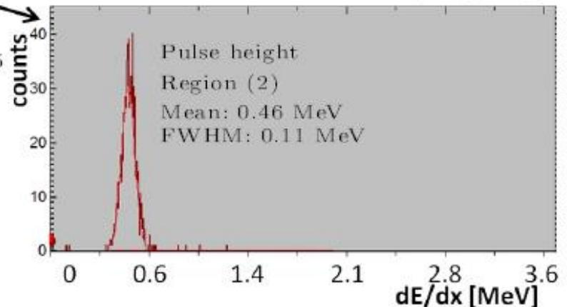
→ pulse height spectrum reduced by a factor of 5.1 at absorbed dose of about 87 MGy
