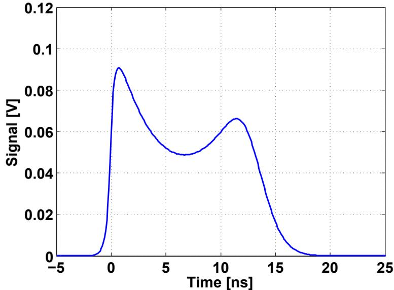
Simulated TCT pulses for electrons
