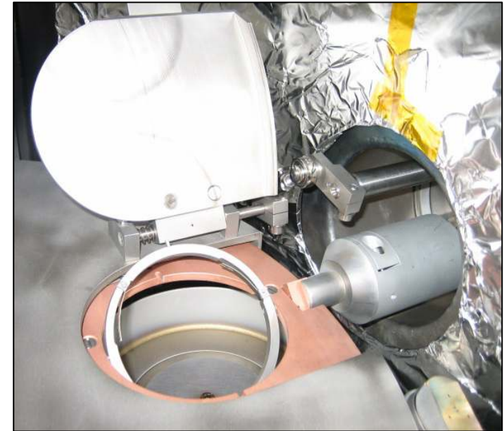
rotatable substrate holder with 10 positions
