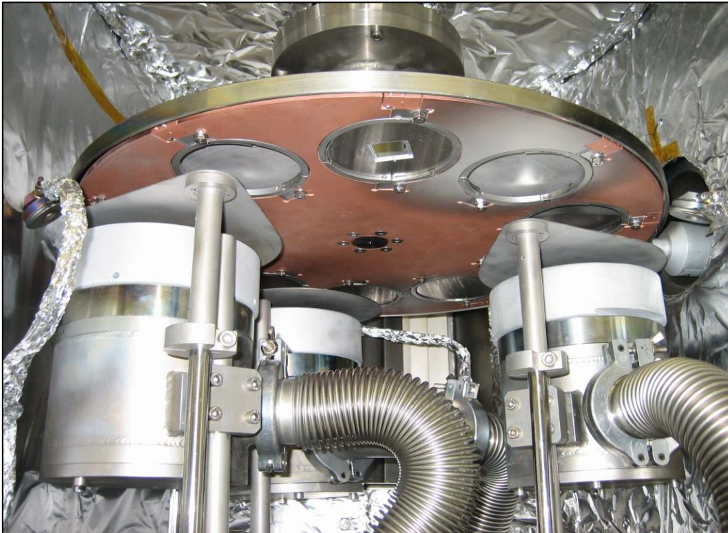
rotatable substrate holder with 10 positions
