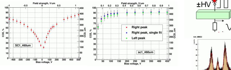
Presence of pumping effect was checked by irradiating the sample with Sr source for ~ 12 hours (~1-2Gy)
