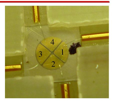
Bonding to Al metallisation problematic We were able to properly contact only MFDia886-2 And only with conductive glue
