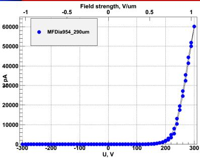
Current spike corresponds to increased noise, CCE measurements are difficult above 250V
