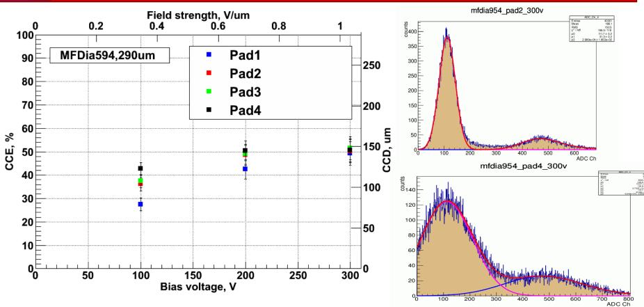
There is some difference in CCE between the pads But the saturated CCE value is ~ 50% for all pads High noise is only visible for pad 4
