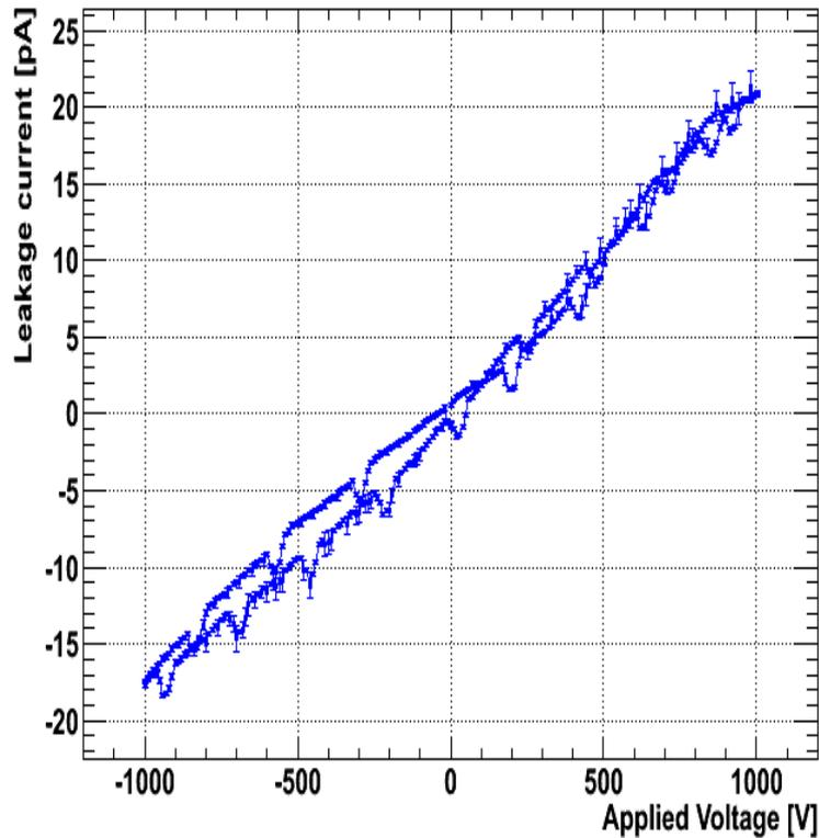
Si leakage  $4.4e15$  protons/cm<sup>2</sup>
