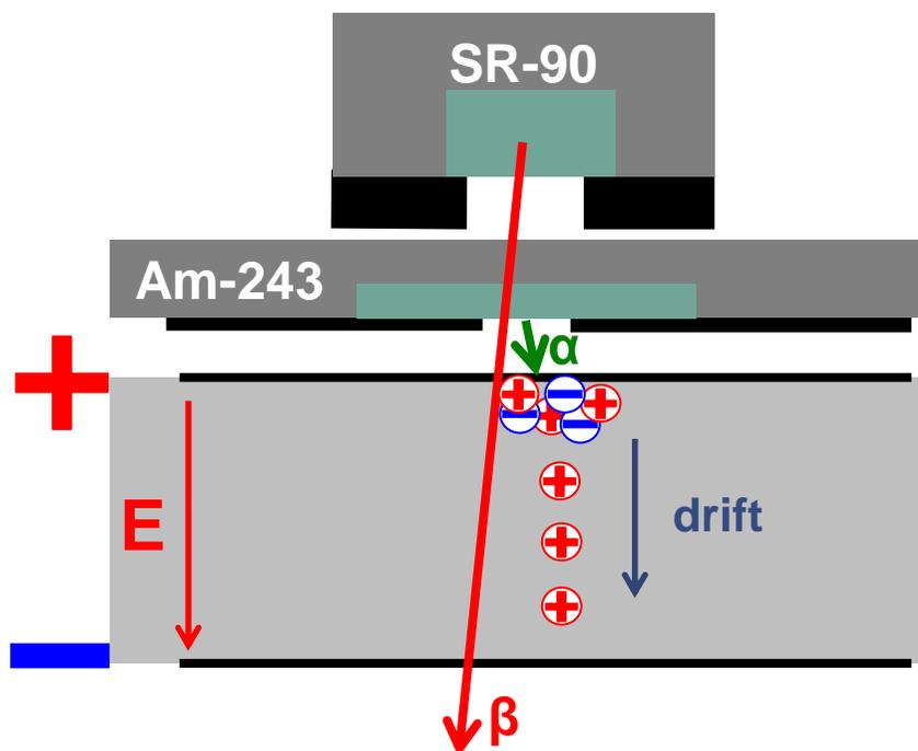
sCVD diamond, 200V, hole drift, with Sr-90 source for polarizing
